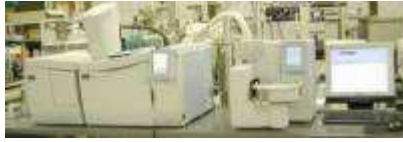
Gas Chromatograph with fully integrated Mass Spectrometer detection system and thermal desorption sample station
